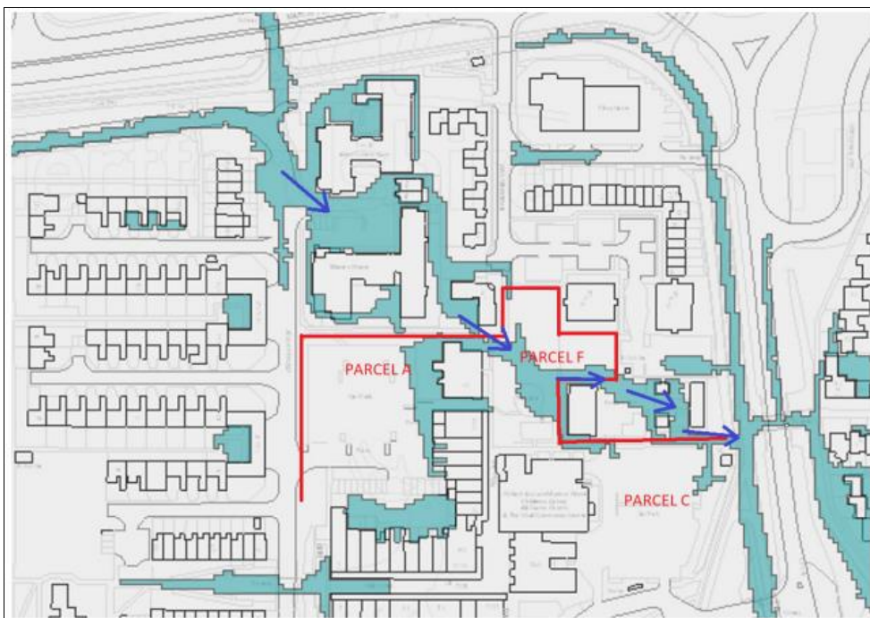
Figure 7 Surface water flow paths
